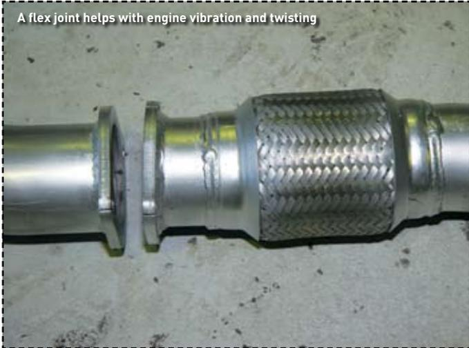
A flex joint helps with engine vibration and twisting
