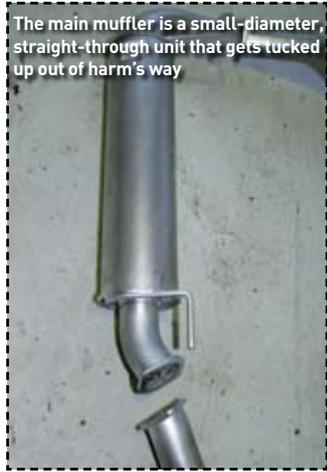
The main muffler is a small-diameter, straight-through unit that gets tucked up out of harm's way
