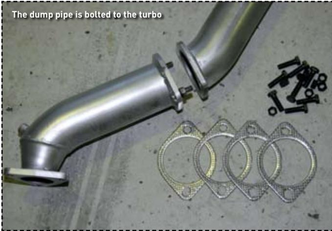
The dump pipe is bolted to the turbo
